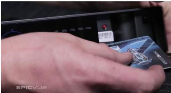
The card goes right in the slot behind the access door on the front of the receiver unit. There's an arrow showing which direction to insert the card.
