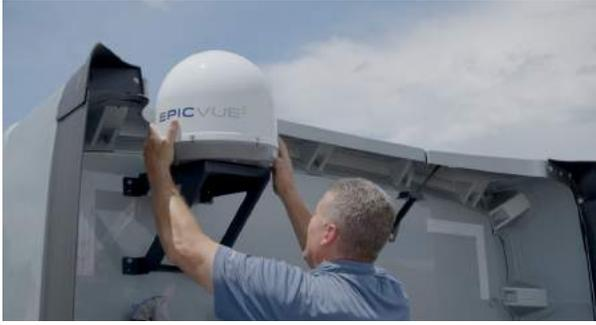
**8.** Now it's time to put the EpicVue satellite dome on the bracket. There are multiple sets of mounting holes on the Top Pivot Plate. Use the set of holes that allows you to get the dome as close to the truck as possible. Fairing extensions or other obstacles may necessitate using the outer set of holes.
