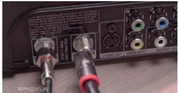
Now install the power plug included with the AC power box into the power port on the left side of the power box and plug the other end of the cord into your power strip.
