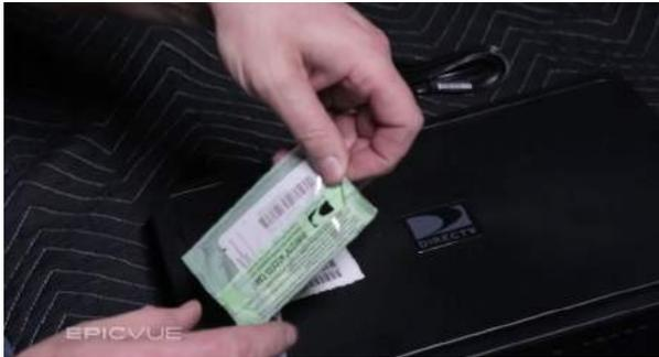
**1.** The receiver comes packaged in a box with the power cord and access card. You want to be careful not to discard this access card. Sometimes the access card is taped to the top of the receiver in a little green tinted package or is already installed in the card slot located on the front of the receiver.
