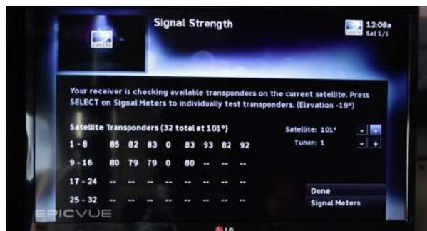
If numbers are showing up under most of the transponders, then select Done, and it will go back to the previous screen. Just verify that 01: Round Dish 18", None, Multi-switch and Dual are still showing. Then select continue.
