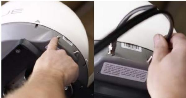
**1.** Apply a small dab of dielectric grease to each coaxial connector on the 29' Dual Coaxial Cable, then connect the coax with the **white writing** on it to the **main** port on the dome. Connect the other coax line without writing to the secondary port of the dome.
