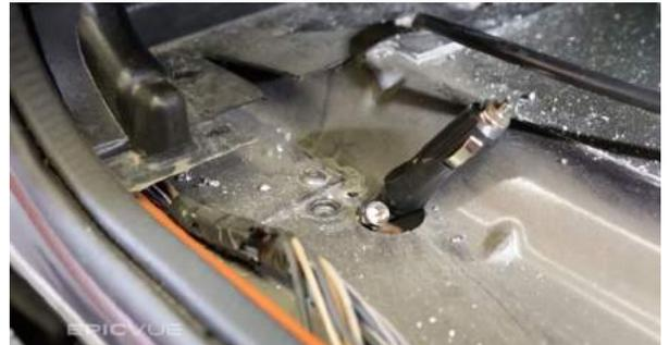
Add about 6" - 8" of flex tubing around the cables at the entry point to prevent them from rubbing and shorting out. Use a zip tie or two underneath the sleeper to prevent the coax from hanging down and catching on something.
