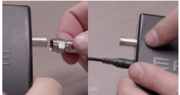
Now connect the other end of the small jumper coax to the outside port labeled Input 1 on the back of the DirecTV receiver.
