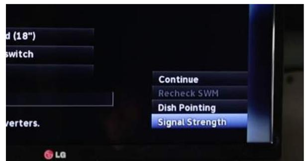
7. If a bunch of zeros show up on this screen, then check connections, and determine why there is no signal from the dish to the receiver. Make sure there are no obstructions between you and the southern sky.
