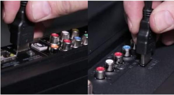
**3.** Next, simply hook up the receiver to the TV. Run the HDMI cord from the TV HDMI slot into the HDMI slot on the DIRECTV receiver.
