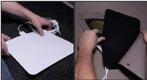
**1.** This antenna is usually placed in the top window and secured between the window and the window shade. Then run the cables down to the cabinet and down to the rear of the Direct TV receiver.
