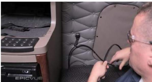
**3.** Once you have run the cables into the cab, pick a route to run the cables to the entertainment center.
