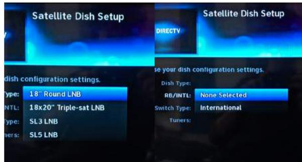
5. This is the critical part of the receiver set up. On the dish type, select 01: Round Dish 18". Below that is the RB/Intl, Select "None".
