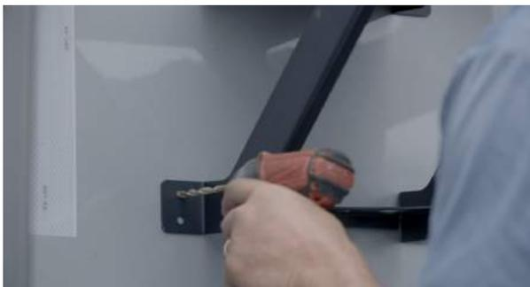
**3.** Next, start the other corner and drill a 1/4" pilot hole and then use another 1/4"-20 bolt in that hole to temporarily hold the bracket up so we can finish drilling the remainder of the holes. This technique eliminates the use of a paper template as well as another person to help-out. Use at least 6 of the holes on the 2 piece bracket to properly secure the bracket to the truck. Use all 8 holes on the 1 piece bracket to properly secure the bracket to the truck.
