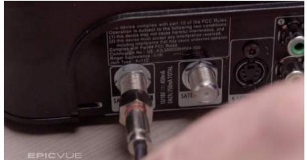
Connect the other coax cable coming from the secondary port on the dome to the inside port labeled Input 2 on the back of the DIRECTV receiver. Finger-tighten these connections, then secure them with a 7/16" end wrench so the vibration from the truck won't loosen them.
