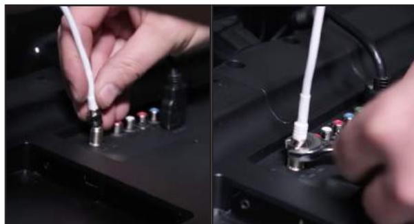
**3.** Connect the coax cable on the end of the antenna to the antenna in port on the back of the TV. And tighten that down, and then secure with a 7/16 end wrench.
