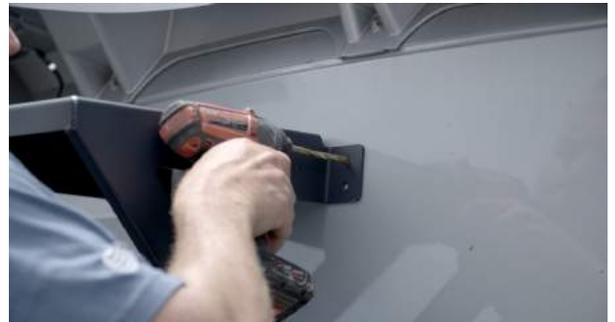
**\*Be aware during installation, the ground that your truck is sitting on may not be level so it's best to use the lines of the truck rather than an actual level to visually level the bracket.**
