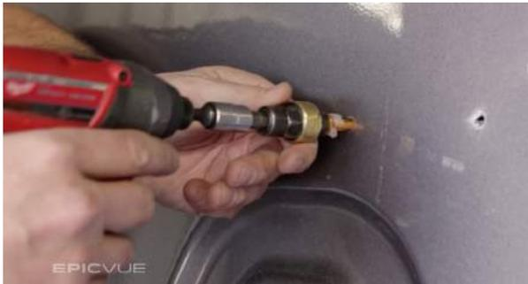
**5.** Using an impact gun with between 1100 to 1300 inch-pounds and the 3/8 Hex bit with the Riv-nut tool, twist one of the Riv-nuts on the end of the Riv-nut tool mandrel.
