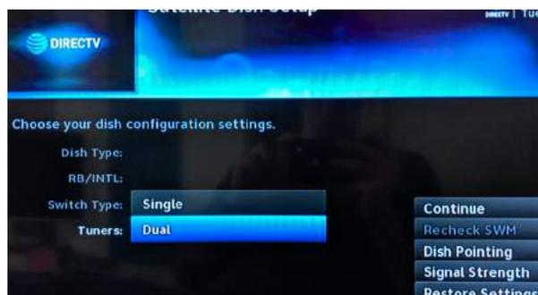
Double check that the tuner type is set to Dual Tuner. Do this so the driver can watch one show, while recording another..
