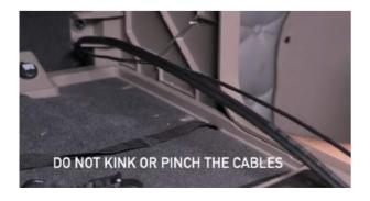
Choose a path that has little disruption and minimal alterations to the current configuration. Whatever you do, do not put the cables in a location where they could potentially get kinked or pinched. This will prevent satellite signal from reaching the receiver, and you will not get any picture.
