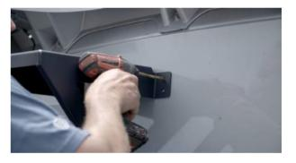
\*Be aware during installation, the ground that your truck is sitting on may not be level so it's best to use the lines of the truck rather than an actual level to visually level the bracket.
