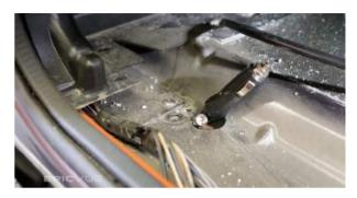
Add about 6" - 8" of flex tubing around the cables at the entry point to prevent them from rubbing and shorting out. Use a zip tie or two underneath the sleeper to prevent the coax from hanging down and catching on something.
