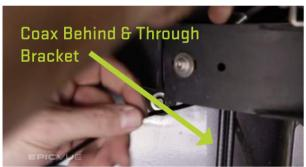
Feed this coax across the sleeper and down through the wind-fairing brackets.
