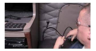
**3.** Once you have run the cables into the cab, pick a route to run the cables to the entertainment center.
