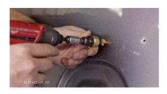
5. Using an impact gun with between 1100 to 1300 inch-pounds and the 3/8 Hex bit with the Riv-nut tool, twist one of the Riv-nuts on the end of the Riv-nut tool mandrel.
