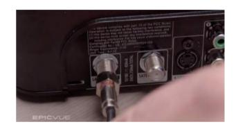
Connect the other coax cable coming from the secondary port on the dome to the inside port labeled Input 2 on the back of the DIRECTV receiver. Finger-tighten these connections, then secure them with a 7/16" end wrench so the vibration from the truck won't loosen them.
