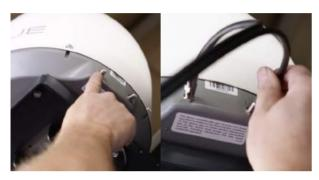
1. Apply a small dab of dielectric grease to each coaxial connector on the 29' Dual Coaxial Cable, then connect the coax with the **white writing** on it to the **main** port on the dome. Connect the other coax line without writing to the secondary port of the dome.
